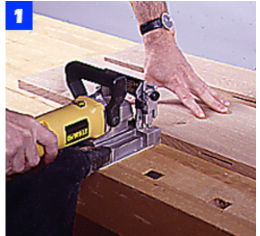
1 Cut and joint stock for the sides, top, bottom, partition and shelves. Then cut slots in mating edges with a plate joiner.
