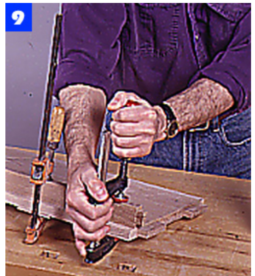
Join the bottom front rail to the case bottom with joining plates and glue. Clamp together until the glue sets.
