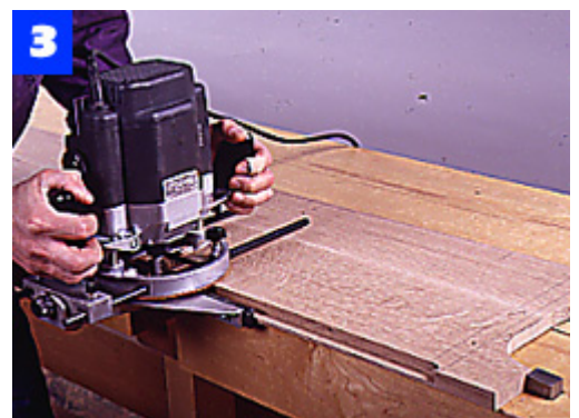
3 Cut the rabbets for the back panel in the case sides and top using a router with a 3/4-in.-dia. straight bit and edge guide.
