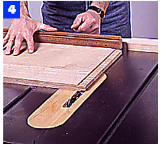
Use a table saw with a dado blade installed to make the tenon cuts on the ends of the case bottom and top.
