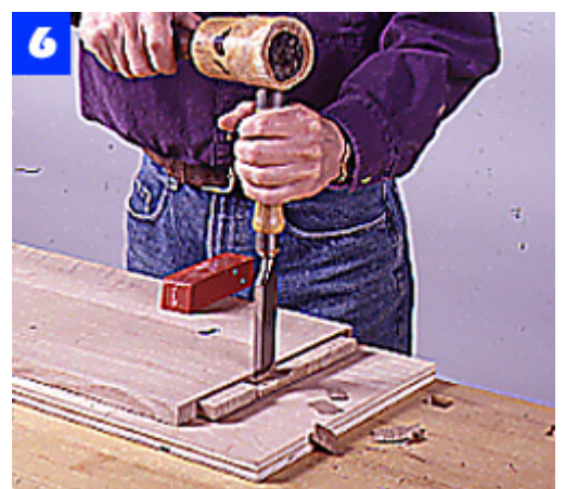
Use a chisel to remove waste between the through tenons. Work from both sides of the board to prevent tearout.
