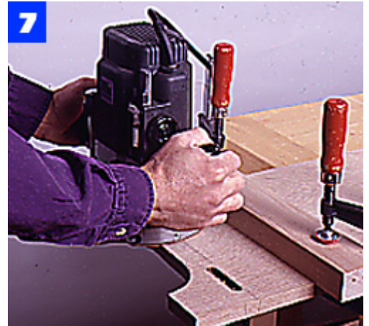
Cut the through tenon mortises in the case sides using a router with an up-cut spiral bit. Square the cuts with a chisel.
